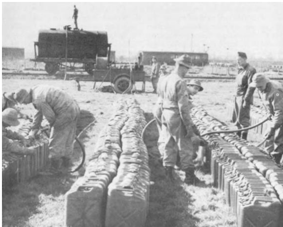
Filling 5-gallon fuel cans at a DTC railhead
